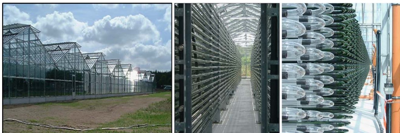
Fig. 3 A high-end closed bioreactor system. The worlds largest closed photo-bioreactor in Klötze, near Wolfsburg, Germany (Bioprodukte Prof. Steinberg; www.algomed.de ); the 700 m 3 are distributed in 500 km of tubes and produce up to 100 t algae biomass per year
